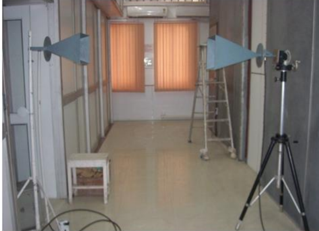
Fig: Reference Level Measurement Setup At 2100 MHz at outside chamber
