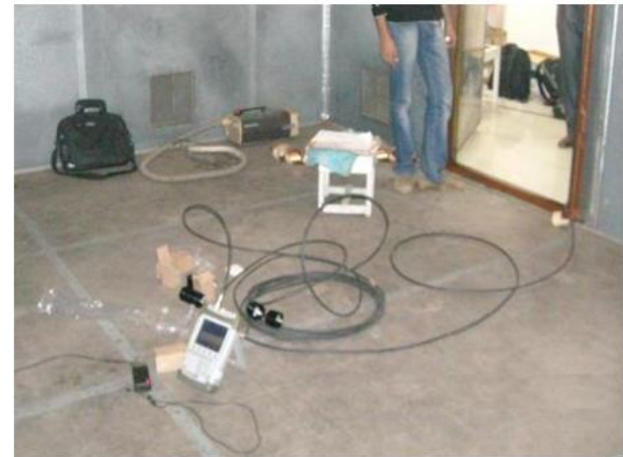
Fig: Reference Level Measurement Setup At 900 MHz at inside chamber
