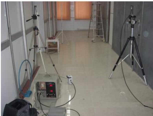
Fig: Reference Level Measurement Setup At 900 MHz at outside chamber
