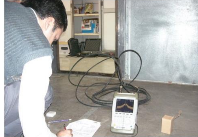
Fig: Reference Level Measurement Setup At 2100 MHz at inside chamber
